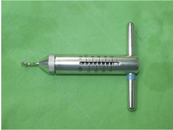
Fig 1. Tensiometer for measuring repair tension of the rotator cuff.
